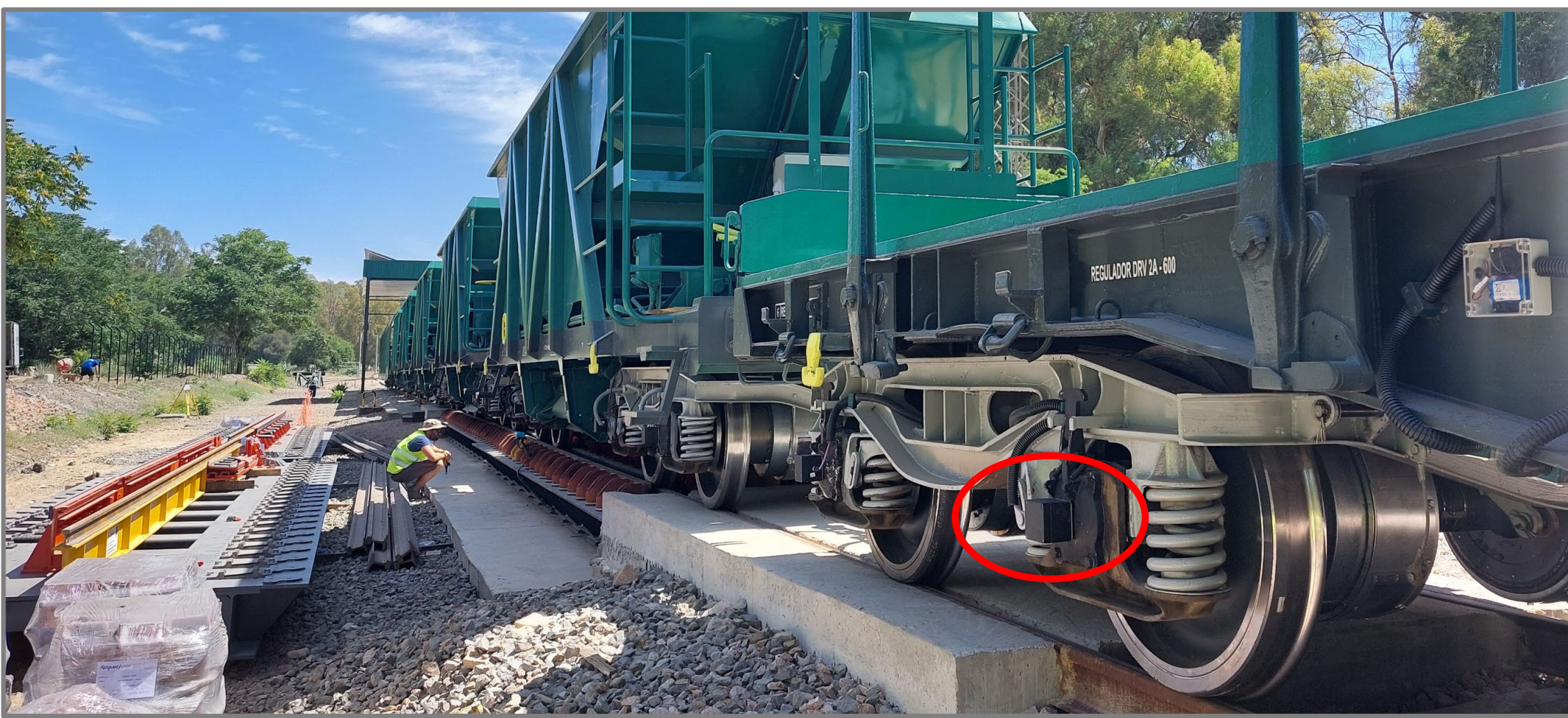
(****) Acceleration, temperature and position sensor
