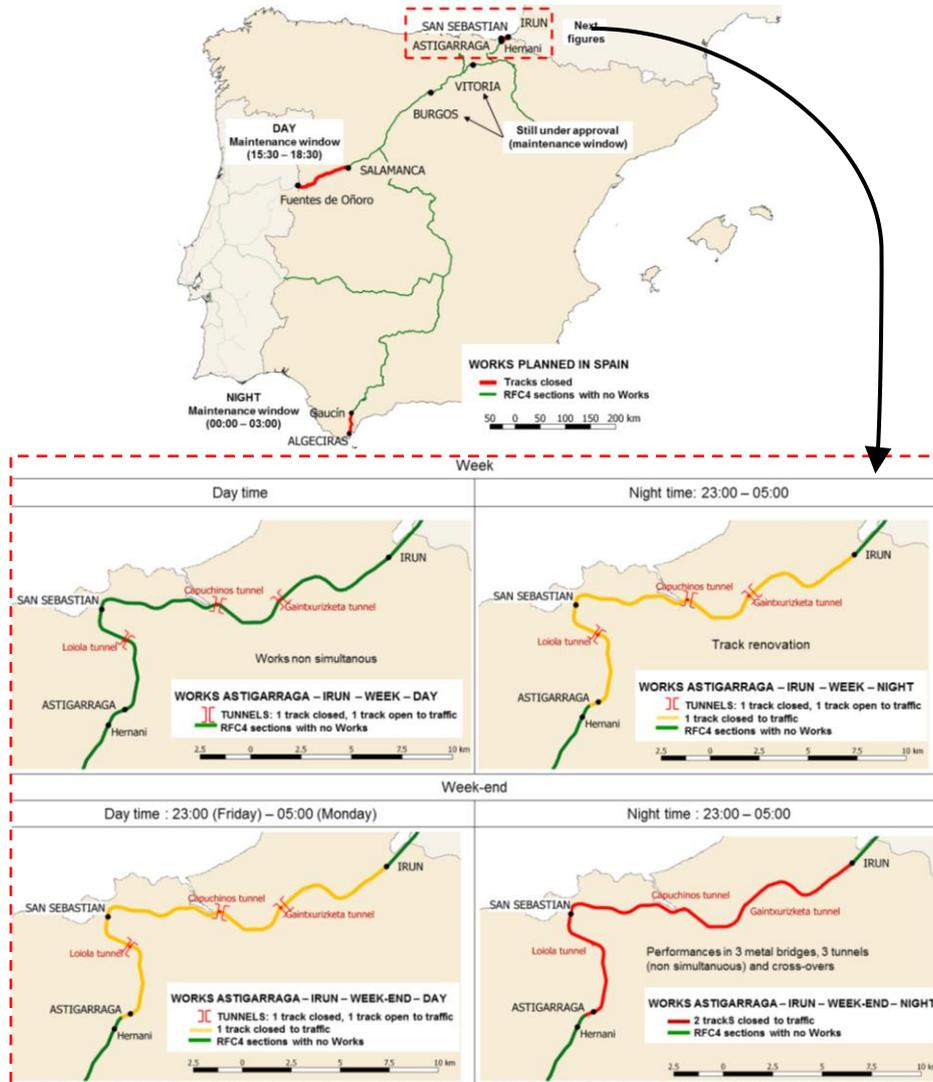
Figure 2: Works planned in Spain along the RFC4. Source: IDOM elaboration
