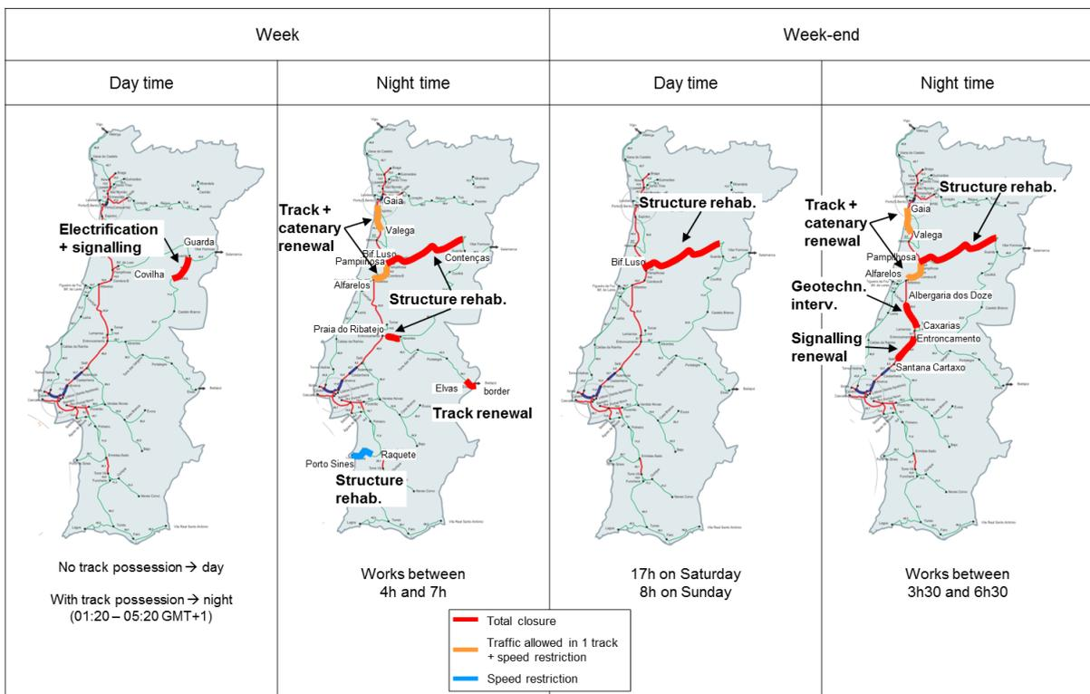
Figure 1: Works planned in Portugal for 2017. Source: IDOM elaboration
