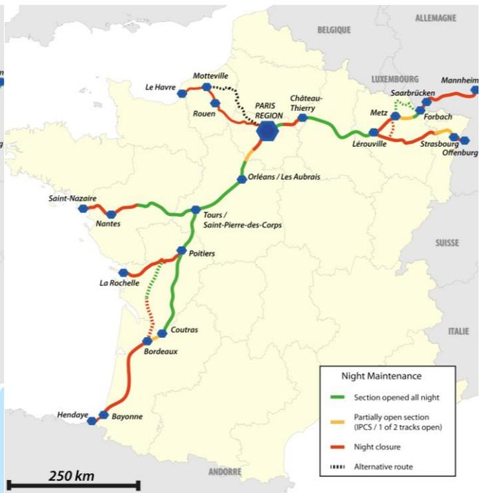
Figure 7 : Night maintenance along RFC4 in France and Germany. Source: ARCADIS elaboration
