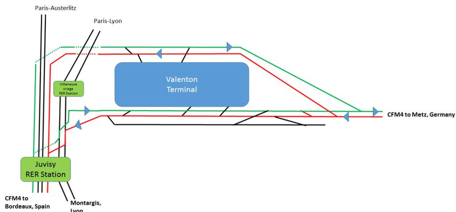
Figure 11: Valenton Access Terminal (source ARCADIS / SNCF RESEAU)
