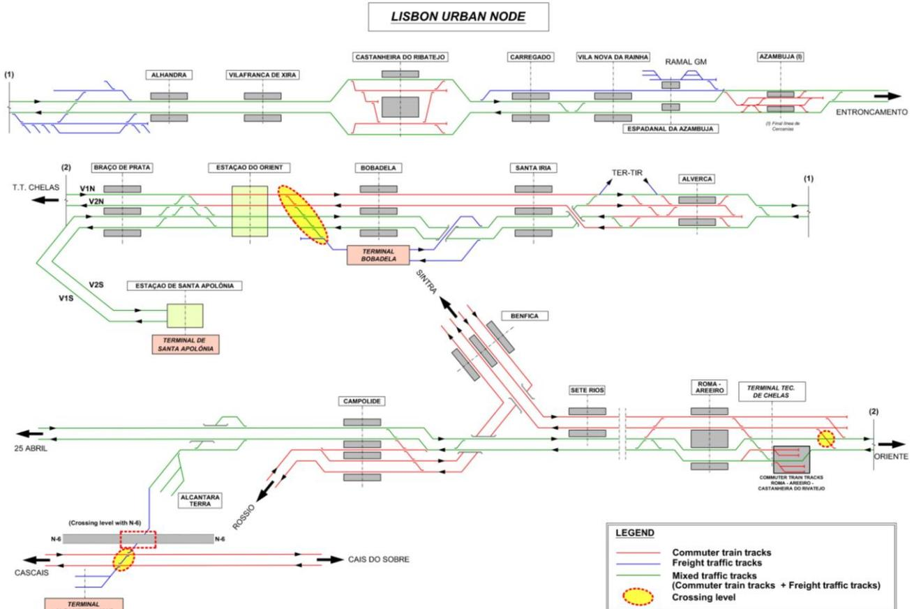
Figure 8: Functional scheme of rail infrastructures in Lisbon urban node. Source: IDOM elaboration
